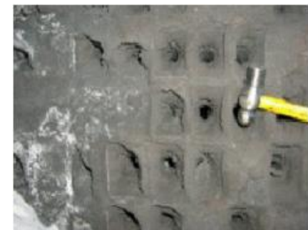
Syngas Cooler plugged
