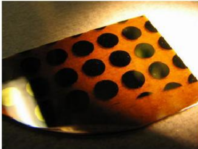
CO 2 splitting semiconductor/catalyst device under construction (gallium phosphide wafer with metal contacts) Credit: Aaron Sathrum, UCSD
