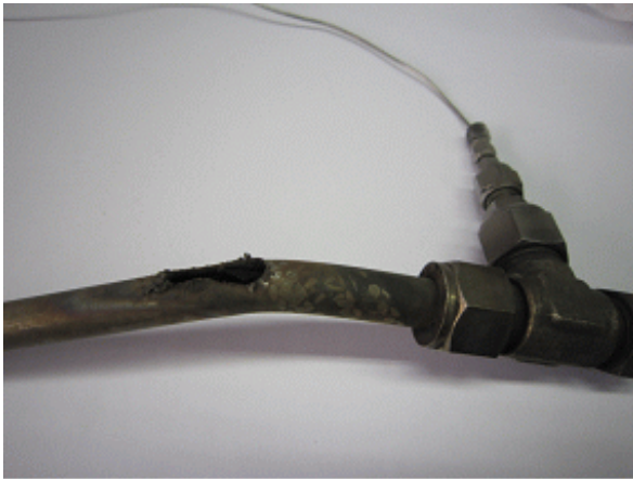
Damaged SUS coal powder feeding pipe occurred at the 8 bar and around 1,500°C gasification pilot plant test.
